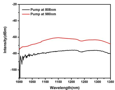
Figure 3. Luminescence spectra of PbS/PbSe co-doped fiber excited by different pump light source.
