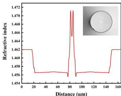
Figure 1. Refractive index distribution curve of the PbS/PbSe co-doped fiber, (inner) cross section of the fiber.
