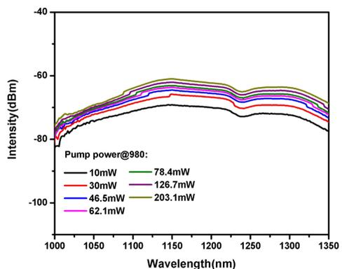
Figure 4. Luminescence spectra of PbS/PbSe co-doped fiber under different pump powers.
