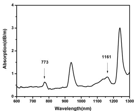
Figure 2. The absorption loss spectrum of the PbS/PbSe co-doped optical fiber.
