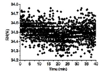
Fig. 6 Graph of the calculated RH versus the time over 40 minutes when RH's fixed at 34.5%.
