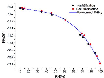
Fig. 2 Plot of the PR versus the RH roughly ranging from 10% to 100% in the humidification and dehumidification process
