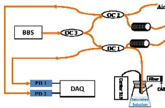
Fig. 1 The overall differential Fresnel reflection based humidity sensing system.
