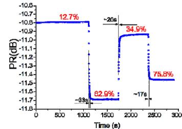
Fig. 5 Real-time response of the proposed differential Fresnel reflection based humidity sensor
