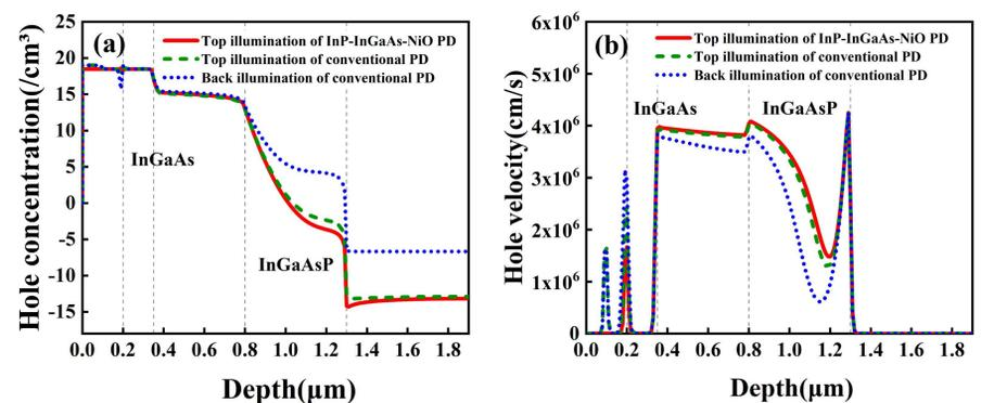
Figure 4. (a) The hole concentration (b) hole velocity of different photodetectors in the radial direction.
