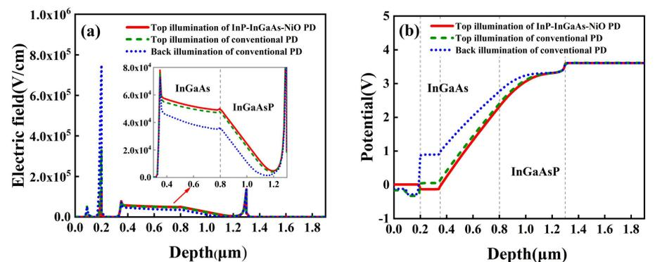
Figure 3. Distribution of (a) electric field and (b) potential of different photodetectors in the radial direction.
