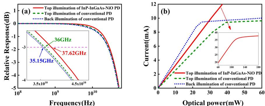
Figure 2. (a) The bandwidth (b) the DC saturation current of different photodetectors in different illumination methods.
