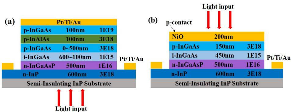
Figure 1. The epitaxial layer structure of (a) conventional photodetector and (b) InP-InGaAs-NiO p-i-n photodetector.
