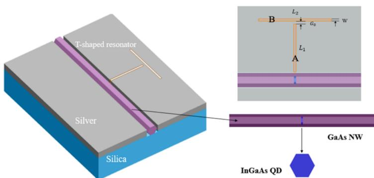
Figure 1. 3D schematic diagrams of InGaAs/GaAs QDNW heterostructure.
