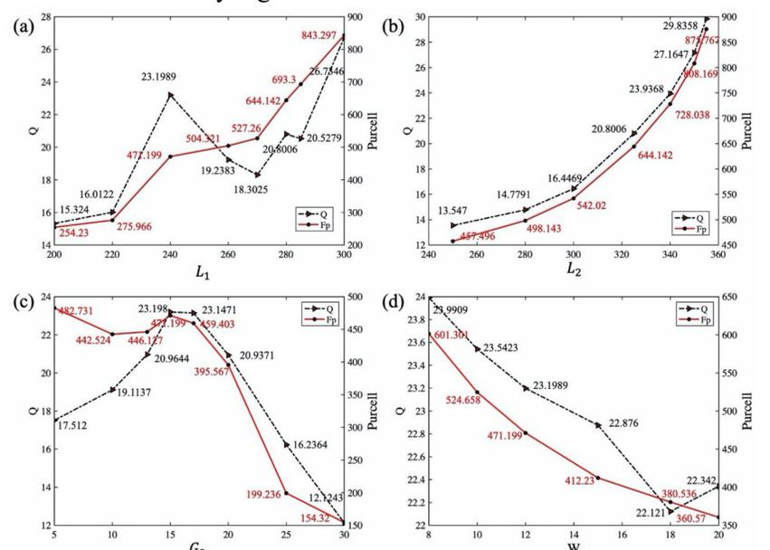
Figure 4. (a-d) Dependence of Q factor and Purcell value on the different parameters.
