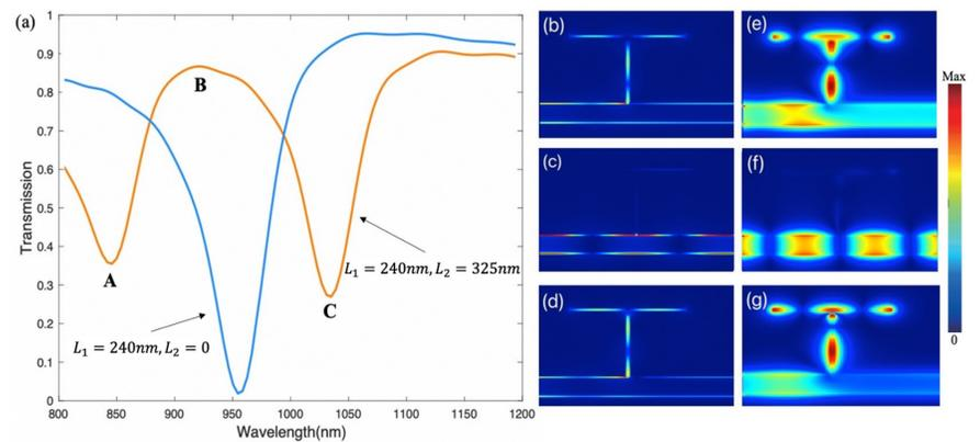
Figure 3. (a) System transmission spectra with or without A resonator. (b-g) Distributions of electric amplitude and magnetic amplitude corresponding to the three frequency values represented by  $f_A$ ,  $f_B$ , and  $f_C$ , in (a).
